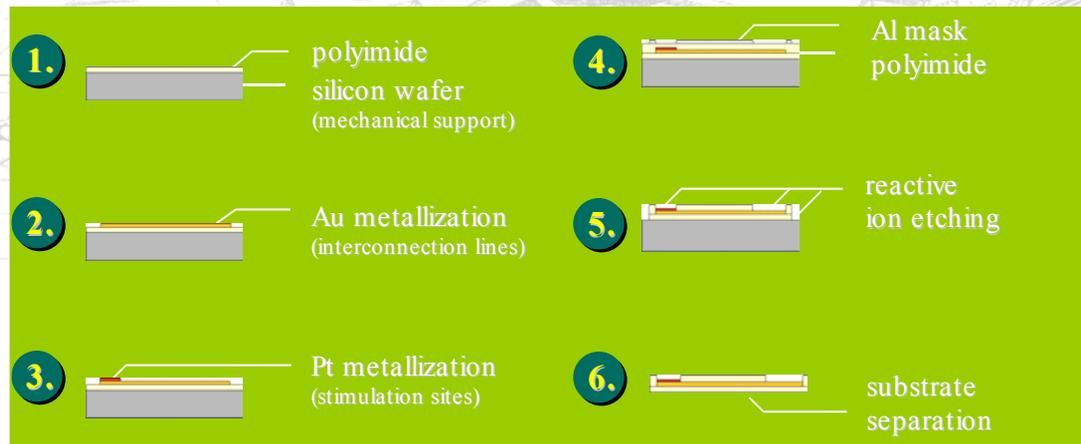
Technology process for the sieve electrodes implementation
