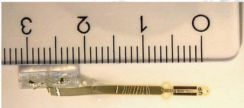
Sieve like electrode with tube and connector
