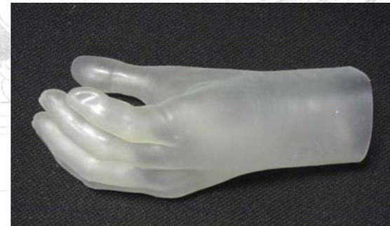
The first prototype of the cosmetic glove has been already fabricated and preliminary tested. The colour and other aesthetic details like nails, hairs, etc. have been not yet added.
