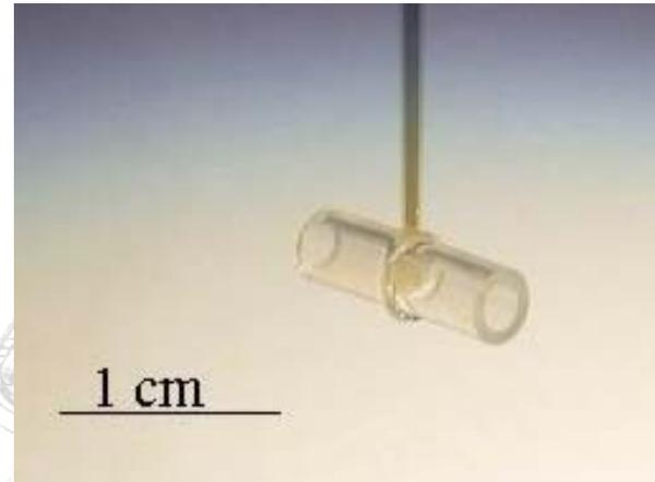
Sieve electrode with silicone tube
