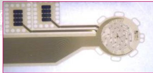
Sieve Head with Counter Electrodes
