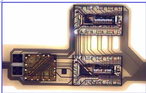
Integrated Electronics for Active Sieve Electrode
