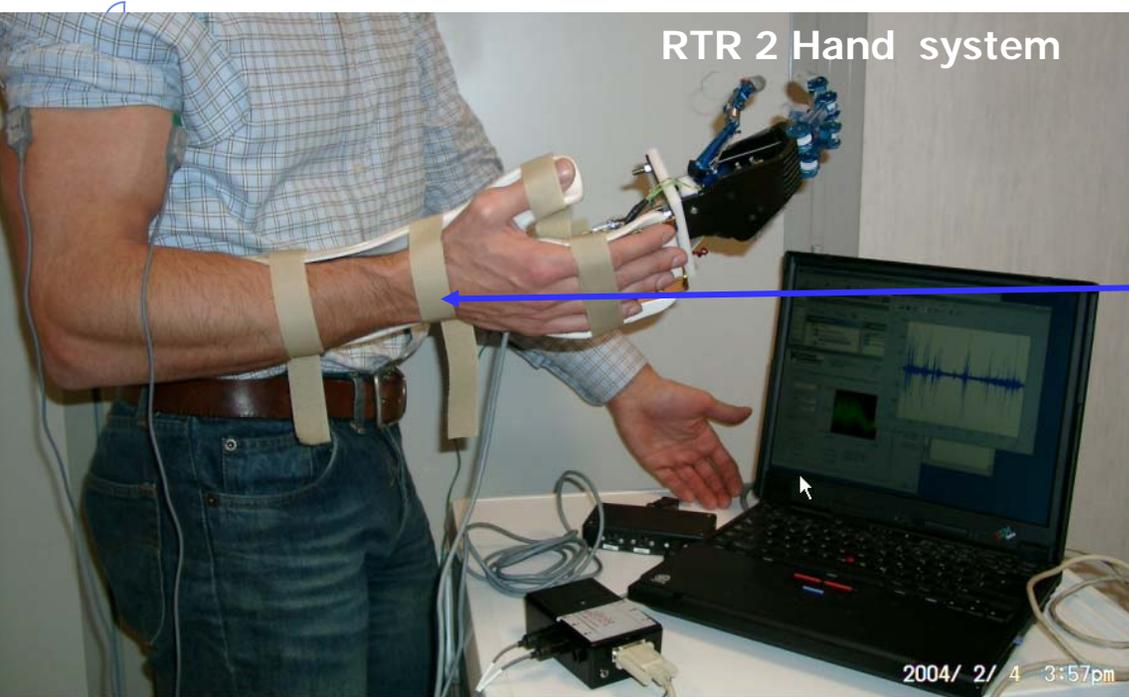
The prosthetic device can be assessed by normal subjects wearing the prosthetic system with a splint
